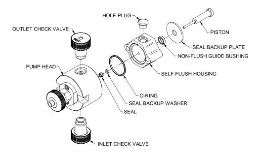
Figure 5-4. Bioclean (PEEK<sup>TM</sup>) Non-Self-Flushing Pump Head Assembly
